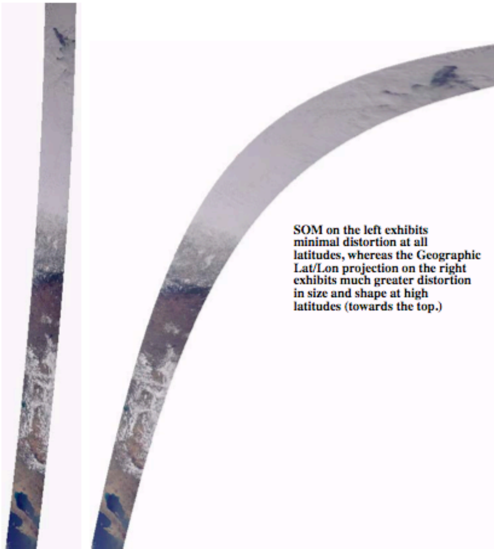
Figure A-3 Sample Partial MISR Swath in SOM vs. Distorted Geographic Lat/Lon
