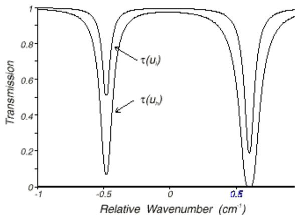
Figure 2. Transmission through a cell with two distinct amounts of the absorbing molecule in the path.
