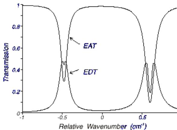
Figure 3. The Equivalent Average Transmission (EAT) and Equivalent Difference Transmission (EDT) of the signals passed through a long and short path of an absorbing molecule.
