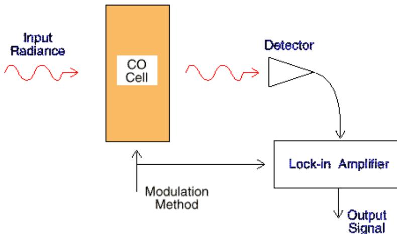
Figure 1. Schematic of a typical Correlation Radiometer (CR).
